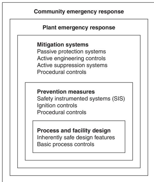
**Figure 5-13.3.** Typical risk reduction layers at industrial facilities.
