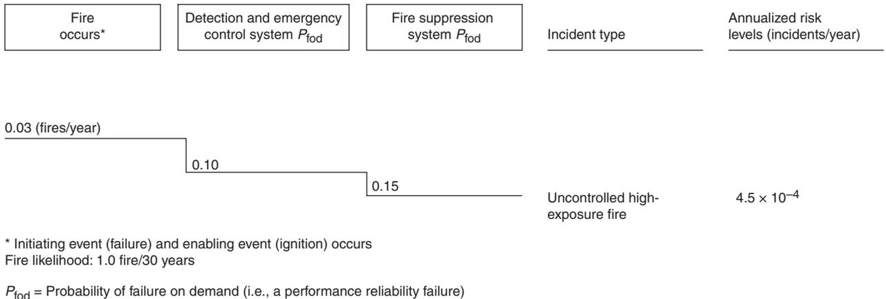
Figure 5-13.6. Example of the correlation between a simple fire event tree and FPS-LOPA.
