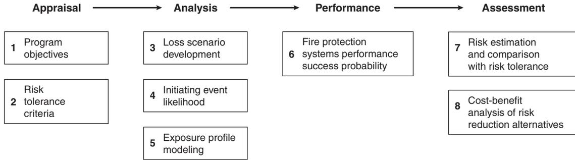
**Figure 5-13.8. Risk-informed performance-based fire protection steps.<sup>1</sup>**
