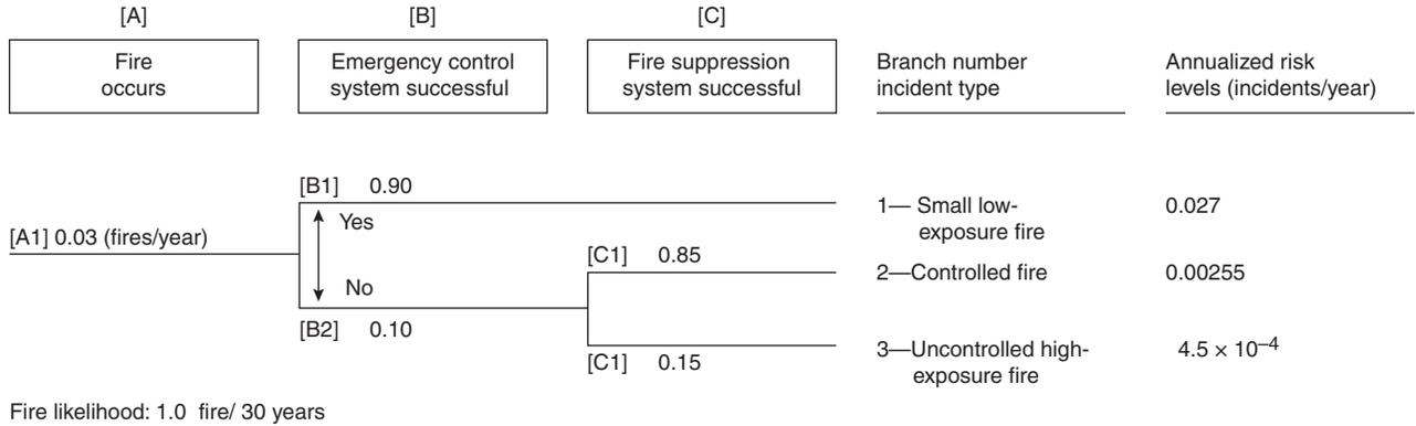
Figure 5-13.5. Example of a simple fire event tree.
